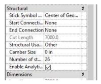
The design info (composite beam design info and virtual joist design info) is available as an attribute of the member. Studs and camber info are imported to Revit as properties of the "Structural frames", Joist designation is imported as "comments" and moments & shear forces at ends are imported into Revit as "Member forces". For Joist girders, in addition to above, the number of spacing and the point load will be updated in the property "SpaceNum" and the Panel poinbt load respectively.
