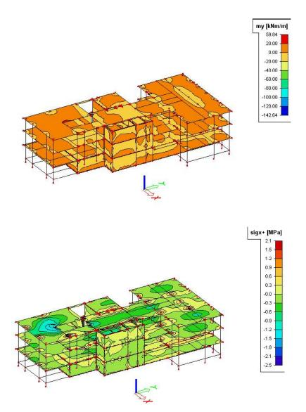
For instance, the size of the two columns shown below is reduced from 200x600 mm to 200x450 in the SCIA Engineer model.
