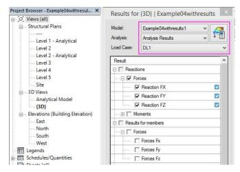
Select the required result type and click on Apply at the bottom of the dialog to view the result.
