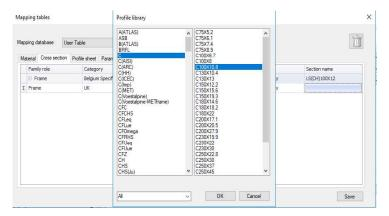
For families which are defined with dimensional parameters, use "document mapping" option. You will not be able to add mapping entries for parameteric sections in the user table directly.
