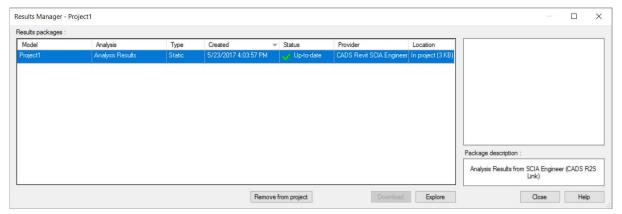
The option to view results is available in the results explorer which can be launched from the review manager by clicking on *Explore* or by directly selecting the *Results Explorer* option in the *Analyse* tab under *Structural Analysis* group.
