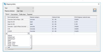
Revit materials in the document will be listed based the material class and SCIA Engineer materials will be listed based on the National code.
