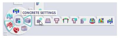
For the calculation of the reinforcement an effective depth is needed which is based on diameter and cover. The concrete cover and diameter can be set separately for both the upper and lower face of the slab. For walls there is only one setting available that is applied to both sides.
