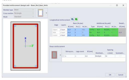
This means that in the provided reinforcement we always have the basic reinforcement of 2 bars – on the upper and lower edge – of diameter 16mm. This can be increased with the values of the additional reinforcement. However, this will only be increased if the provided reinforcement is less than the required reinforcement. This comparison will be done for each section of the beam.
