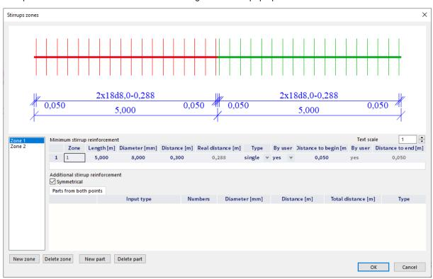
Currently we have two zones over the full length of the beam. We can create a new zone by first making the current zone shorter. Instead of the full length of 10m we will choose 2,5m for this zone. Then we can make new zones of 5m and 2,5m:
