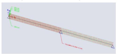
The practical reinforcement is added as reinforcement data. You can edit the reinforcement by selecting it and then click on 'Edit reinforcement'.
