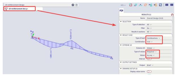
You can access the template of the theoretical provided reinforcement of the member by using the action button 'Edit provided reinforcement template' and selecting the member:
