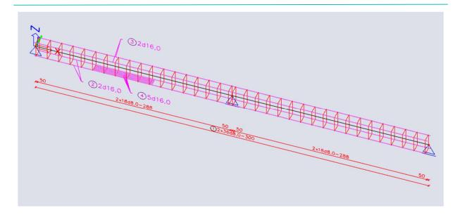
The next step is to change the shear reinforcement. First, select the shear reinforcement. Then, choose 'Edit stirrups distances' under Actions and the following window will pop up:
