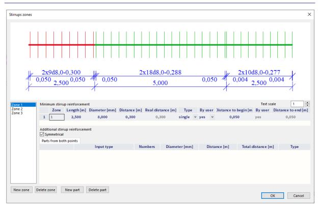
Now we can adjust the distances for each separate zone. For example: Zone 1 = 0,1m; Zone 2 = 0,2m; Zone 3 = 0,3m:
