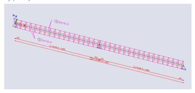
We can also adjust these zones of reinforcement if necessary, by selecting them and changing the parameters in the properties window. However, in this case we want to add the 4 bars of diameter 16 to the middle of the first span. Therefore, we need to choose 'New longitudinal bars' and choose the length of this new zone. We will input the bars over a length of 2m:
