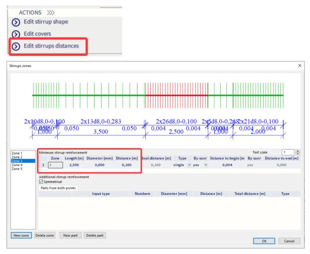
By selecting the reinforcement, it is always possible to change the parameters afterwards through the property window.
