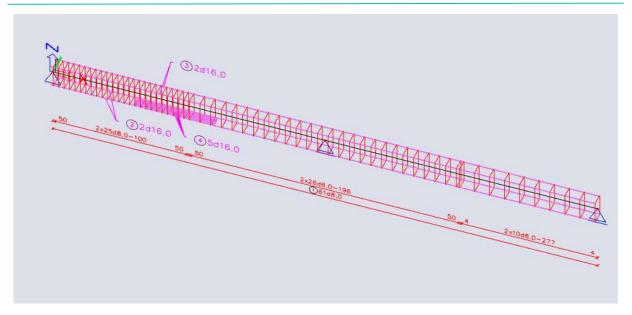
Finally, after all necessary adjustments are made and the practical reinforcement is inputted, this can be used to perform the 1D checks.
