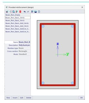
This template exists of basic, additional and shear reinforcement. The purpose is to compare these templates with the required reinforcement, to model the user reinforcement that is introduced later or to convert it automatically to user reinforcement.
