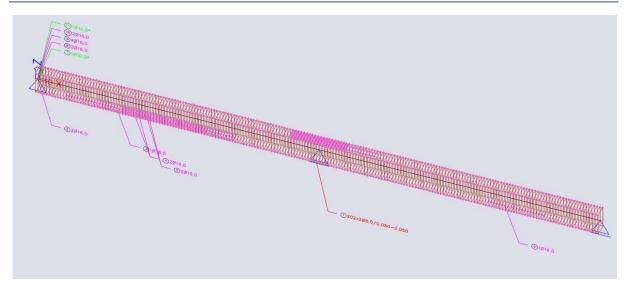
Here we see the basic reinforcement of 2 bars of diameter 16mm along the full length of the beam. On section dx=2.5m we now have the increased reinforcement of 5 bars of diameter 16mm which is of course coming from additional reinforcement inputted in the template of the provided reinforcement. The values of 1 bar of diameter 10 is the detailing reinforcement that is required to meet the detailing provisions. The shear reinforcement is also presented along the length of the beam.
