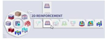
You can add reinforcement of any kind onto the slab. To take into account this information in the calculation of provided reinforcement, enable the below option in the result properties:
