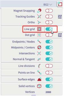
Search for "Opening on 2D" in SCIA Spotlight and create the first opening by choosing "New circle (By center & radius pt.)" underneath the SCIA spotlight, snapping on the grid lines and typing "@0,01 0 0" in the SCIA Spotlight to define the radius.
