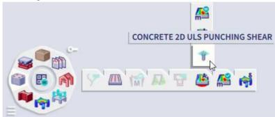
This check can be executed based on required (theoretical), provided and user reinforcement.
