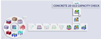
This check can only be executed when there is user reinforcement present in the concrete.
