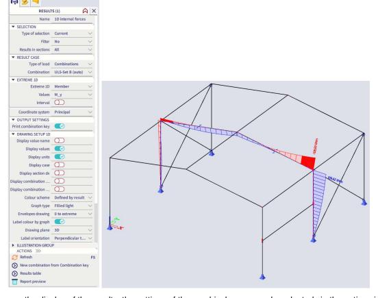
To change the display of the results, the settings of the graphical scene can be adapted via the options in the group **Drawing setup 1D** in the property panel. You can display units, change the colour scheme or graph type, ...
