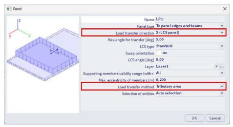
Use the snapping points in the roof to create a load panel for each pitch of the roof.
