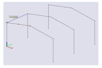
Enter the other beams of the roof in a similar way, always by clicking the top nodes of columns or inclined beams. Add a beam as well at half of the height of the first right span.
