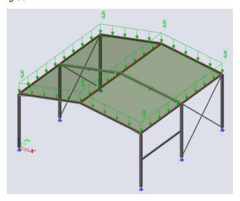
When you calculate the model, the loads will automatically be converted from surface loads to line loads.
