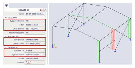
The graphical scene shows that the maximum unity check occurs for one of the middle columns. To understand the reason behind it, you can open the **Report preview** with a detailed representation of the performed steel check. You can find all input data, calculated resistances, code formulas and notices and warnings in the detailed output that usually contains a few A4 pages.
