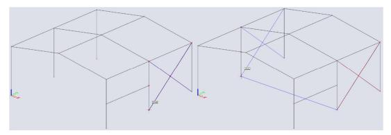
When the members are copied, the command remains active until you press **<Esc>**, so that you can copy as well to other positions if needed.
