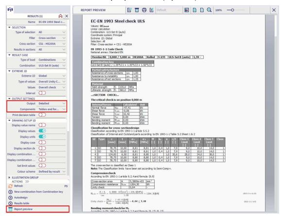
This detailed report reveals that the column does not comply with the **Bending and axial compression check** according to EN 1993-1-1 article 6.3.3 and formula (6.61),(6.62). In this particular project; a different cross-section with larger inertia is required.
