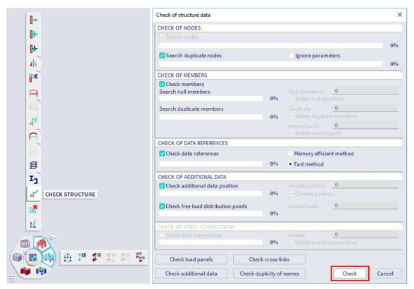
In the **Check of structure data** dialogue the different available checks are listed. Click **[Check]** to perform the checks.
