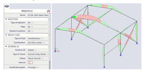
With this check the relative deformations are compared with the deflection limits, as defined in the steel settings or via the system lengths and buckling settings. When the check is exceeded, you can check if the deflection limits are set properly or you need to change the cross-section of the elements. An SLS autodesign command is not available in SCIA Engineer.
