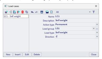
We will create a second permanent load case for the roof weight. Click on [New] and change the **Description** to **Other permanent loads**. The **Load type** is now set to **Standard**.
