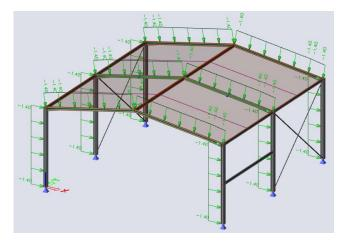
Select the linear loads on the roof girders and the columns of the first and last frame by clicking with the left mouse button on these loads. The mentioned members must have only half of the load value because only half of the loading width, affected by wind, belongs to them.
