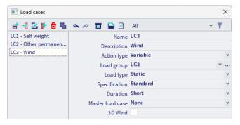
The **Load type** determines the composition factors (psi-factors) that are attributed to the load cases in this load group. In this project choose **Wind**.
