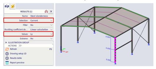
You can ask as well for the slenderness (Lam y or Lam z), buckling factor (ky or kz), buckling length (ly or lz),... The buckling length is determined as the reference length multiplied by the buckling factor.
