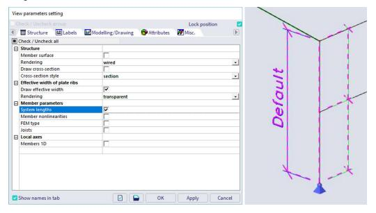
The figure above shows that the (default) system/reference length **Ly** (blue line) for buckling around the strong axis (y-y) is the total height of the column and **Lz** (green line) for buckling around the weak axis (z-z) is half of the height. The girder in the middle of the column therefore supports the column for buckling around the weak axis.
