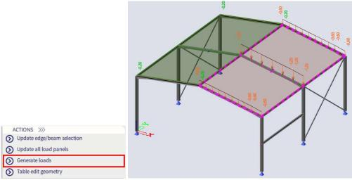
Go to the **view settings** and switch on the tab **Loads/masses** the **Generators** to **Generated** or **Original + Generated** if the loads remain green. Or use the toggle in the View bar.
