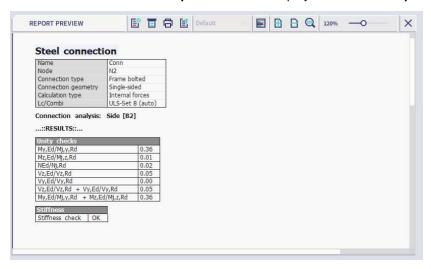
You can set the **Output** as **Brief**, **Summary** or **Detailed**. The summary output shows the internal forces, design resistances, results of unity checks and moment-rotation diagrams.
