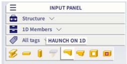
As indicated, a haunch requires a cross-section with a possibility to create variable dimension(s). Since this project does not contain any variable profiles yet, the **New cross-section** window automatically appears.
