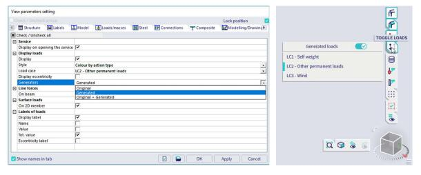
In the **status bar** change the active load case to load case LC3.
