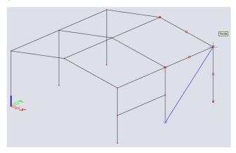
Repeat selecting start nodes and end nodes to model both bracings at the right side.
