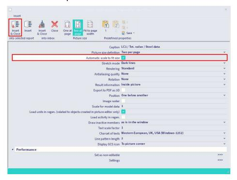
In the report you can indent this item under the item Load cases. When regenerating this item, an image will automatically be generated for each load case (in case that **Selection type** is set to **All** in the properties of the load cases item), based on the image that you have added before.
