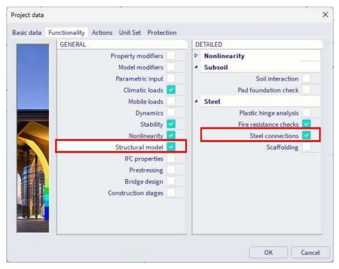
In the analysis model, the members arrive in the same node. But in practice the girder is cut for instance at the column flange or vice versa. You can indicate this through the structural model.
