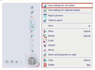
Through the tab **Structure** the representation of the different entities can be adapted
