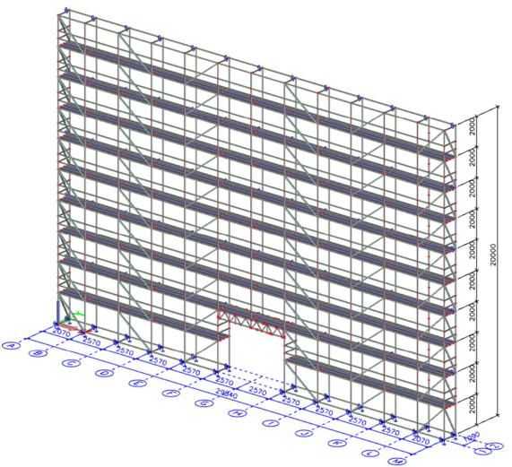
After modelling the structure (elements, couplers, supports, nonlinearities, ...), adding the loads and calculating nonlinearly we can perform the checks on the beams and the checks on the couplers.
