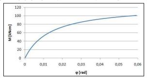
According to this curve, a nonlinear function My is linked automatically to the coupler:
