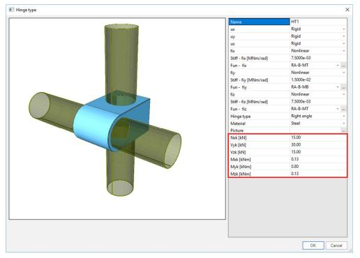
The rigidities and maximal forces are taken from the code EN 12811-1 Annex C Characteristic values of the resistances for couplers.
