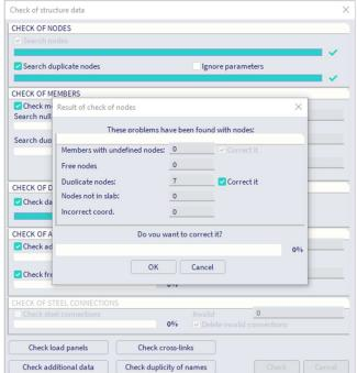
Run the Check structure command to eliminate the duplicate nodes at the top:
