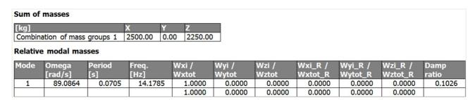
The calculated modal damping ratio is shown to be 0,1026 or 10,26%.
