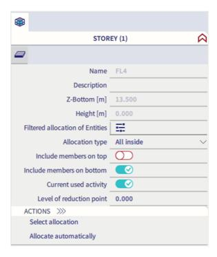
You can check if the supporting members of the building are properly allocated to storeys using the 'Filtered Allocation of Entities' property.
