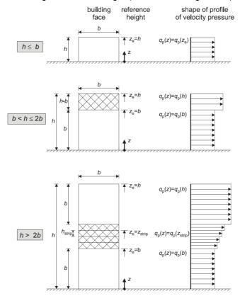
In the example discussed in this course, the height is 20 m and the building face is 29.84 m. So in this case clearly 20 m  $\leq$  29.84 m and thus h  $\leq$  b. So the wind only has to be calculated for  $z_e$  = 20 m.
