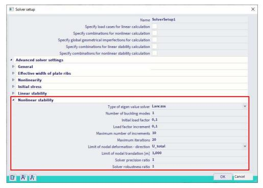
You can start with 1 or 2 buckling modes and evaluate if a global mode is found. If not, you can increase the number of buckling modes or you can change the element that is too weak.
