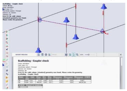
This is because on the right side, the element B9 has been connected to the ledger, and not to the standard.
