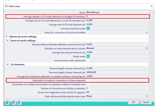
When this option is activated, beams will be connected by the nodes they are going through. But when 4 nodes are inputted on the beams, it could happen that a node has been inputted in the middle of a diagonal and another diagonal is crossing this one in the program and now they are connected. To avoid unwanted connections, we advise to uncheck this option.
