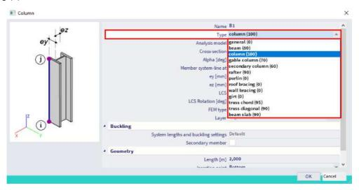
In case two columns are found, both need to be within one buckling system:
