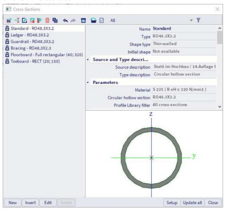
In you want to use a cross-section which is not present in the Profile library (e.g. the floorboard), you can use the group **Thin-walled geometric**.
