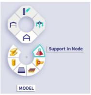
We will add the supports for the **base jacks** (at the bottom nodes of the lowest standards) as nonlinear supports. In the vertical direction these supports can only take pressure and no tension. This is entered in the Z direction with **rigid press only**. The rotations are taken free in all directions.
