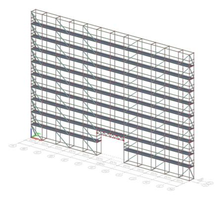
To transfer surface loads to line loads on the beams, we will make use of **load panels** (**Input panel > Workstation Structure > Category Load Panels > Load with load to 1D & edges**).
