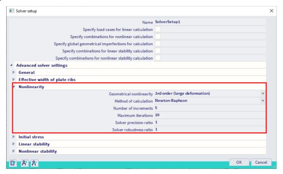
In some cases, a high number of increments may even solve problems that tend to a singular solution which is typical for the analysis of post-critical states. However, in most cases, such a state is characterized by extreme deformations, which is not interesting for design purposes.
