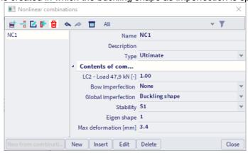
Using this combination, a nonlinear second order calculation is executed using Timoshenko's method.
