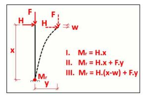
Mathematically, the method is based on a step-by-step augmentation of the load. This incremental method is illustrated on the following diagram:
