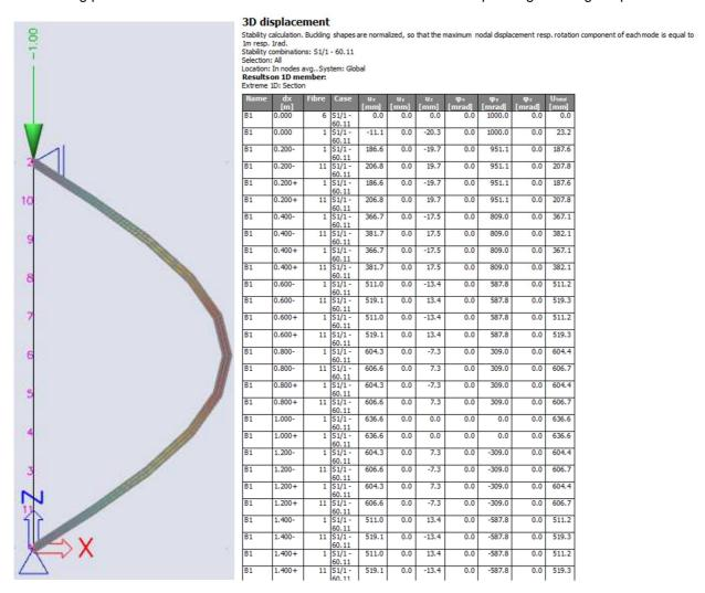
Using for example an Excel worksheet, the buckling shape can be approximated by a 4th grade polynomial.
