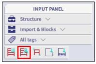
It is also possible to **import** directly from CAD software. To import it you must go to **Menu bar > File > Open from** and choose the desired format (**XML file**, **Revit file**, **Tekla file**, **IFC file**, ...):
