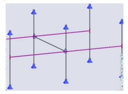
As for the image below, there is an error for the interaction 3 unity check, which states that the geometry is incorrect ("No valid column (standard) geometry was found. Please revise the geometry").
