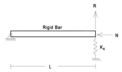
This beam with length  ${\bf L}$  has a pinned support at the left and a flexible spring support at the right with rigidity:  ${\bf K}_{\rm E}$ . Two point loads are inputted on the beam: a vertical force  ${\bf R}$  and a compression force  ${\bf N}$ .
