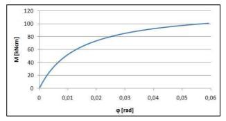
According to this curve, a nonlinear function is linked automatically to the coupler:
