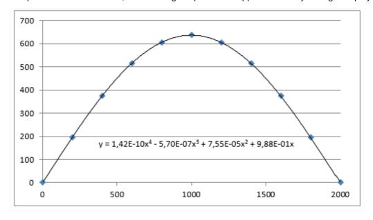
A polynomial has the advantage that the second derivative can easily be calculated:
