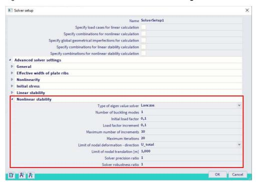
Since the nonlinear stability calculation automatically implies the Modified Newton-Raphson method for the solver, this method cannot be chosen here.
