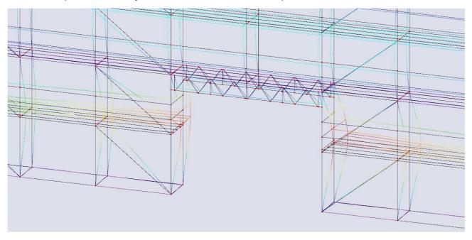
This means we must consider this buckling shape in our nonlinear combinations and analysis.
