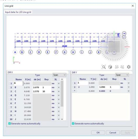
Then we can use the snapping setting **Line grid** (you can find the snapping settings in the status bar) to add the **standards** as column (define the columns as type 'column (100)', 'gable column (70)' or 'secondary column (60)', so the coupler check can be performed later), the **ledgers** as beam and the **diagonals** as member. The standards have a length of 2 m and the ledgers have lengths of 1.09 m, 2.07 m and 2.57 m.
