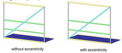
For a ledger of 1.09 m, we will put the floorboards (with a width of 0.32 m) on 0.225 m from the edges of the ledger and with 0.32 m between each other:
