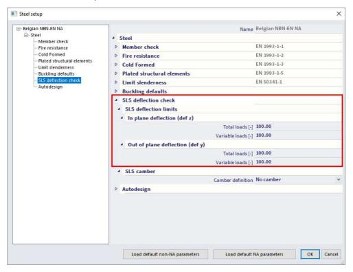
Choose for **Menu bar > Design > Steel members > SLS check** (or **Aluminium > SLS check** in case you have modelled aluminium elements, this functionality is available in the 64bit version since SCIA Engineer 22.0) and ask the results for the nonlinear class **NC\_SLS**:
