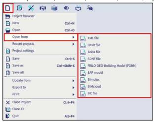
You can also import with the direct links with Revit or Tekla Structures. Even IFC import can be used, but then the model should be cleaned up (align, ...) with the BIM toolbox because with the IFC format we are importing a structural model, which should be converted to an analytical model.
