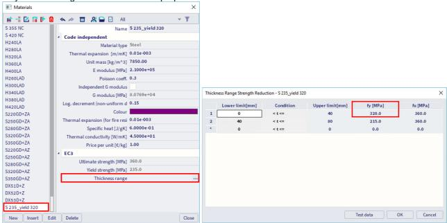
Floorboards can also be inserted as members. The average weight of these elements differs from the weight of material S 235 (due to holes in these elements, another thickness of the elements, ...). That is why it is chosen to insert an additional material in SCIA Engineer, in which the weight will be adapted. This weight can be determined as shown below.
