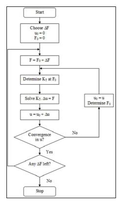
In this figure, the tangential stiffness  $K_T$  is used. The symbol u depicts the displacements and F is the force matrix.
