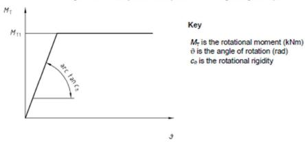
Figure C.2 —  $M_{T^{-0}}$  relationship for class B and C right angle couplers secured by screwed means
