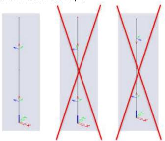
If the above conditions are not fulfilled or if there are more column members found, the column geometry is not recognized and the unity check is set to 999.
