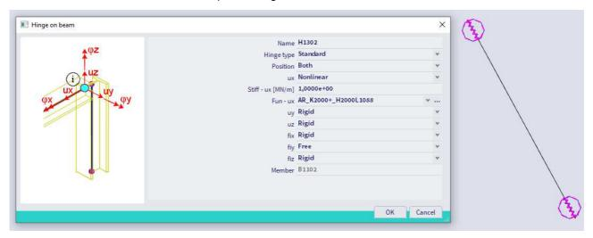
Alternatively diagonals could be modelled via Nonlinearity 1D (Input panel > Workstation Structure > Category Boundary conditions > Nonlinearity 1D). Possibilities are:
