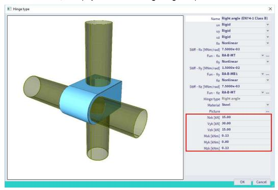
The rigidities and maximal forces are taken from the code EN 12811-1 Annex C. These tables and figures are added in Annex A of this manual.
